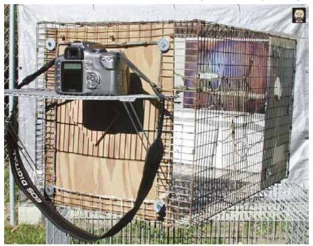
Photobox made from a recycled old cage with camera setup and background in place. Photo ©Richard Renshaw
